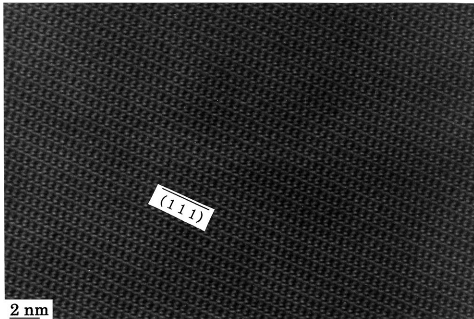
Figure 5 HREM micrograph of \alpha -AlB 12 grain marked by the arrow "C" in Fig. 4A.
