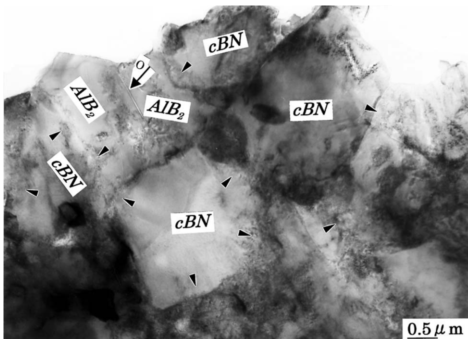
Figure 2 Transmission electron micrograph of the specimen containing 90 mol% cBN sintered under 5.8 GPa at 900 °C for 30 min.
